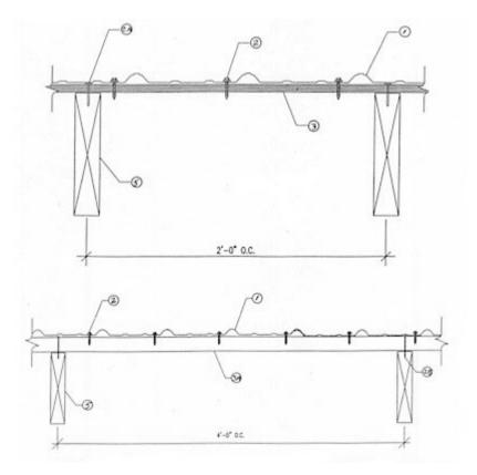
**1. Metal Roof Deck Panels\***-No. 29 MSG min coated steel. Max panel width 36 in. Rib height max 3/4 in. Panels continuous over two or more spans. Panels to overlap 6 in. at endlaps and must occur adjacent to a support when plywood decking (Item 3) is not used. A bead of sealant may be used at panel endlaps and sidelaps.
