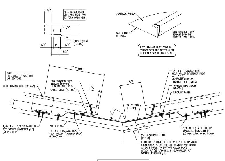
NOTE: DO NOT USE THIS DETAIL ON ROOF SLOPES LESS THAN 3:12 OR IN AREAS W/ SNOW LOADS 10 PSF OR GREATER
