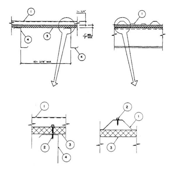
**1. Metal Roof Deck Panels\*** No. 26 MSG min coated steel. Panels continuous over two or more spans. End laps to occur over purlins with panels overlapped 6 in. with lap beginning even with
