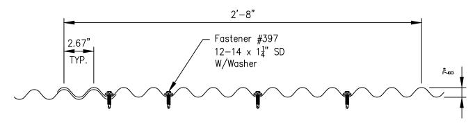
PBC Fastener Location At Intermediate Supports
