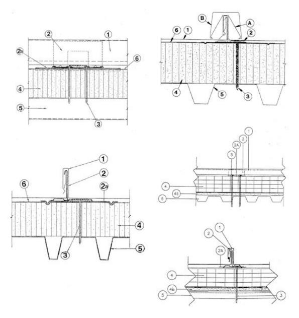
**1. Metal Roof Deck Panels\*** No. 24 MSG min coated steel. Max panel width 18 in., rib height 1-3/4 in. Panels continuous over three or more spans. Endlaps for panels to be overlapped 6 in.
