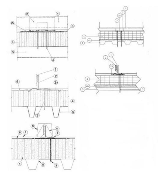
**1. Metal Roof Deck Panels**\* No. 24 MSG min thickness coated steel. Panel width 18 in. max., 10 in. min. ribs height 1-3/4 in. at female side. Panels continuous over three or more clips with no end laps. A bead of sealant may be used at panel side joints.
