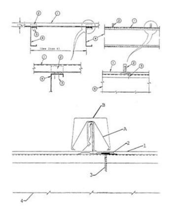
**1. Metal Roof Deck Panels**\* 0.032 in. thick aluminum or No. 24 MSG min thickness coated steel. Panels 10-1/2 in. wide, 1-3/4 in. high at the ribs. Panels continuous over two or more spans. A bead of sealant may be used at panel side joints.
