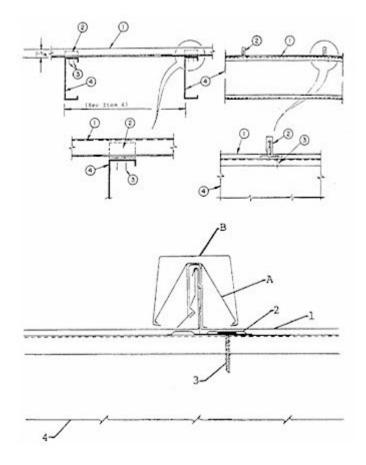
**1. Metal Roof Deck Panels** \* No. 22 MSG or No. 24 MSG min thickness coated steel panels. Panels 12 in. wide, 1-3/4 in. high at the ribs. Panels continuous over two or more spans. A bead of sealant may be used at panel side joints.
