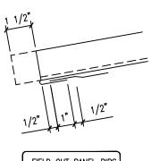
FIELD CUT PANEL RIBS AND BEND PAN OVER TO FORM OPEN HEM
