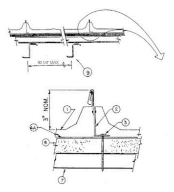
**1. Metal Roof Deck Panels**\* No. 24 MSG min. Coated steel panels continuous over two or more spans. End laps to occur adjacent to purlins with panels overlapped 3 inch max. Side laps to be tightened and crimped with a special motorized crimping machine. A line of sealant may be used at panel end and side laps.
