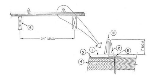
**1. Metal Roof Deck Panels**\* No. 24 MSG min coated steel. Max panel width 22-3/4 in. and rib height 3/4 in. Panels continuous over two or more spans. End laps to occur adjacent to supports with panels overlapped 4 in. A line of sealant may be used at panel ends and side laps.
