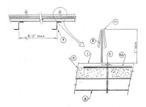
**1. Metal Roof Deck Panels**\* 24 MSG min coated steel. Max panel width 16-1/2 in. and rib height 1-7/8 in. Endlaps to occur adjacent to supports with panels overlapped 4 in. min.
