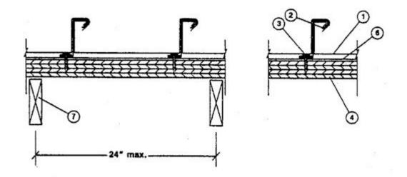
**1. Metal Roof Deck Panels**\* No. 24 MSG min coated steel. Max panel width 16 in., rib height 2 in. Panels continuous over two or more spans. Endlaps to overlap 6 inches. Panels may be physically curved at a radius of 110 ft. or greater. A bead of sealant may be used at panel ends and side joints. Side laps to be tightened and crimped with an electric crimping machine to a min 45 degree angle. Crimping process to include the upper portion of panel clips (Item 2).
