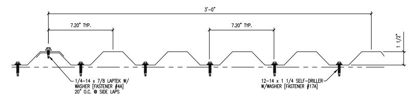
7.2 FASTENER SPACING @ PANEL ENDS & INTERMEDIATE SUPPORTS
