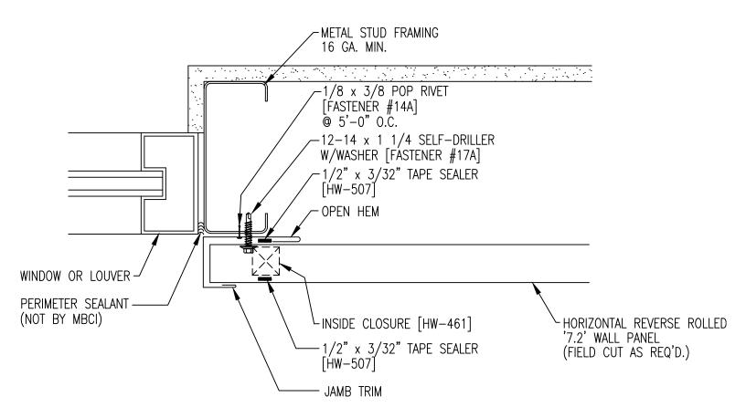
NOTE: MBCI RECOMMENDS THAT A REVERSE ROLLED 7.2 PANEL BE USED IN HORIZONTAL APPLICATIONS SO THAT THE LAP FASTENERS CAN BE INSTALLED IN THE LOW RIBS.
