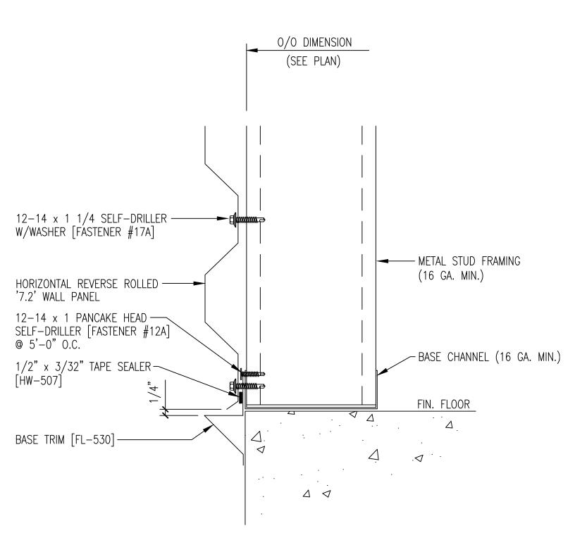
NOTE: MBCI RECOMMENDS THAT A REVERSE ROLLED 7.2 PANEL BE USED IN HORIZONTAL APPLICATIONS SO THAT THE LAP FASTENERS CAN BE INSTALLED IN THE LOW RIBS.
