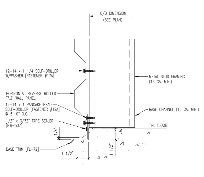
NOTE: MBCI RECOMMENDS THAT A REVERSE ROLLED 7.2 PANEL BE USED IN HORIZONTAL APPLICATIONS SO THAT THE LAP FASTENERS CAN BE INSTALLED IN THE LOW RIBS.
